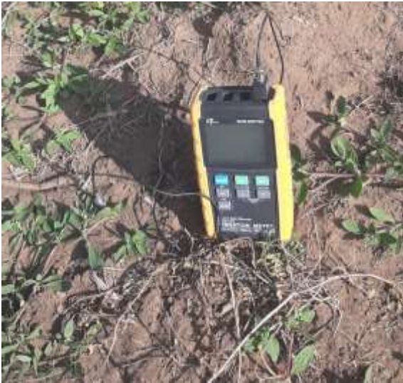
Figure 4-5: Noise and vibration level meters used to collect data on the project site
