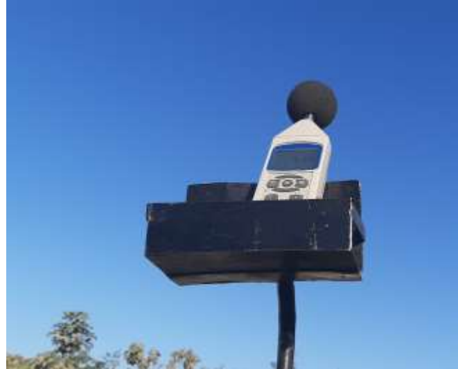
Figure 4-5: Noise and vibration level meters used to collect data on the project site
