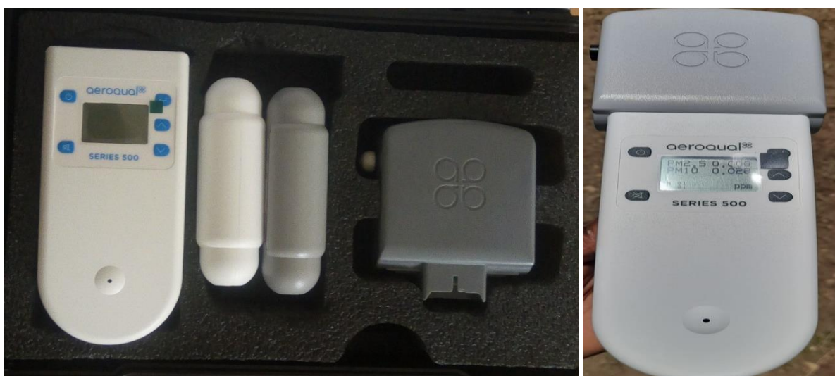
Figure 4-2: Ambient Air Quality Monitoring equipment used at the project
