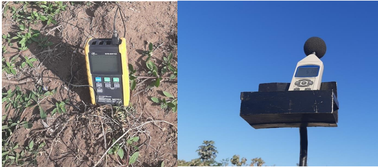
Figure 4-4: Noise and vibration level meters used to collect data on the project site
