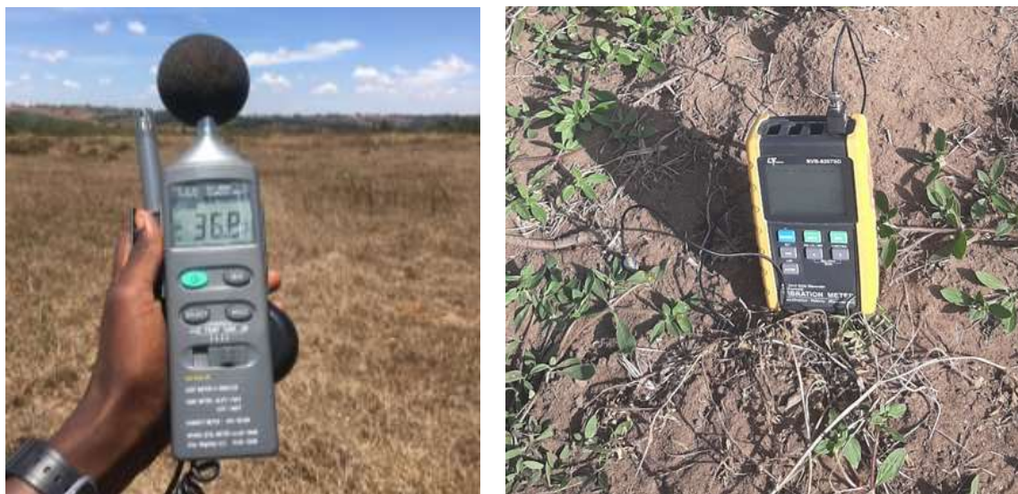
Figure 4-4: Noise and vibration level meters used to collect data on the project site
