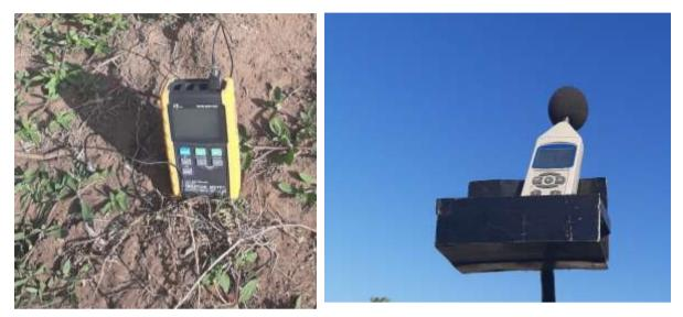
Figure 4-3: Noise and vibration level meters used to collect data on the project site
