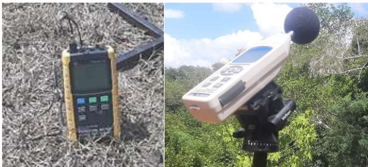
Figure 4-5: Noise and vibration level meters were used to collect data on the project site
