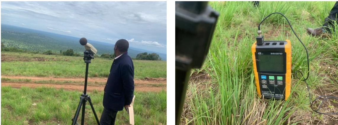
Figure 4-5: Noise and vibration level meters used to collect data on the project site (Tansheq Site Visit, November 2022)
