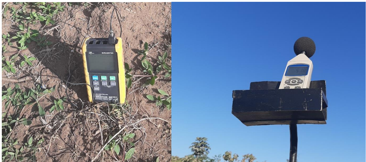
Figure 4-3: Noise and vibration level meters were used to collect data on the project site
